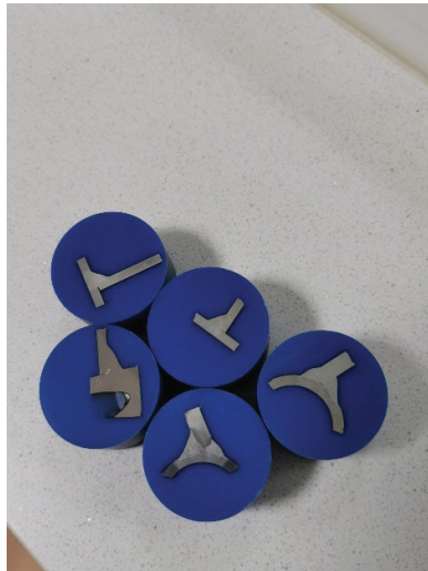
Figure 6: Metallographical samples used for determination of microstructure and microhardness measurements at the single-pass corner welded joints
