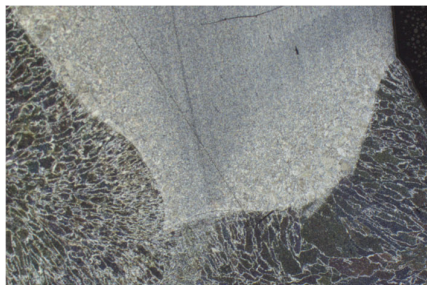
Figure 13 : Microstructure without the presence of cracks in the weld metal, and the HAZ of a single-pass corner welded joint (sample 5, joint 5), mag(50x).
