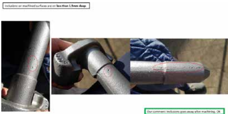
Figure 12: Defects on machining surface [9]
