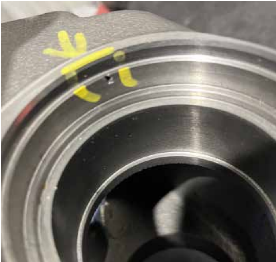
Figure 7: Visible porosity on machined surface [9]
