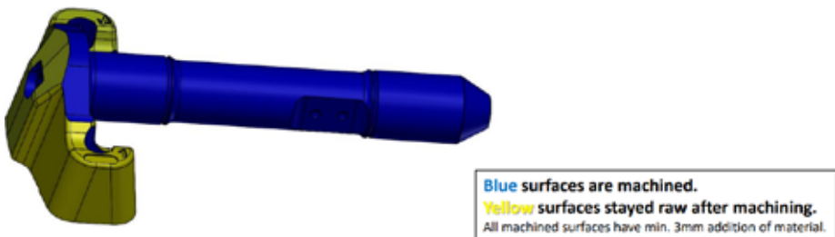
Figure 9: 3D model of a KozolenBoltzen bracket pin sample part [9]
