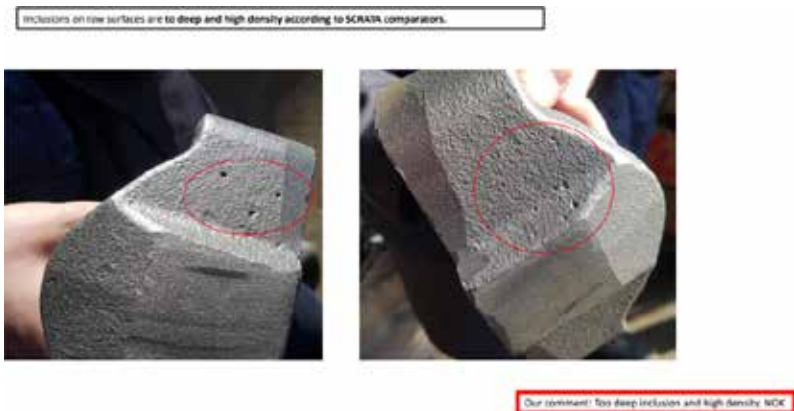
Figure 13: Defects on the machining surface [9]
