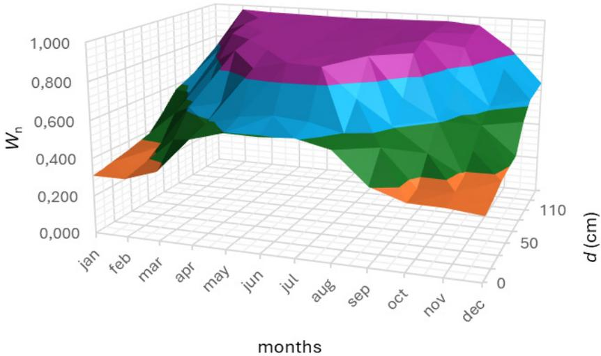
**Figure 5:** Electricity production of the 2<sup>nd</sup> shaded row normalised to the production of the 1<sup>st</sup> row at a tilt angle of 38,5°
