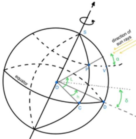
**Figure 1:** Definition of hour angle, latitude and declination [12]
