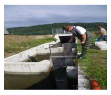
Figure 3: Deployment of a creel in the technical section of the fish pass [8].
