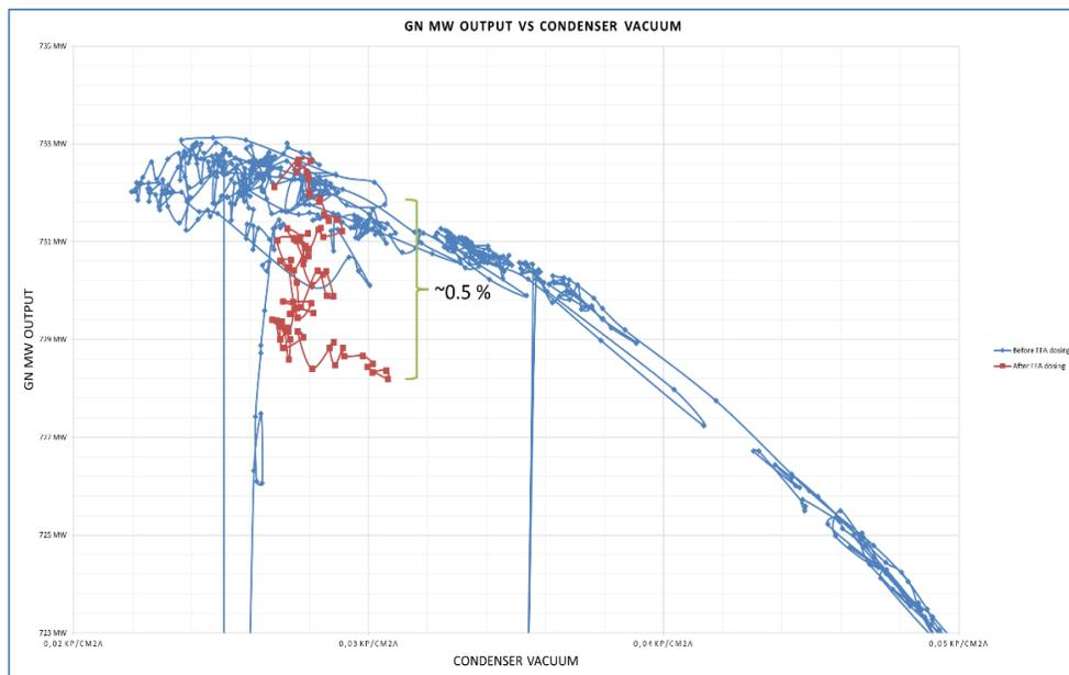
**Figure 4:** The MWe characteristic at the generator relative to vacuum during the addition of FFA chemicals
