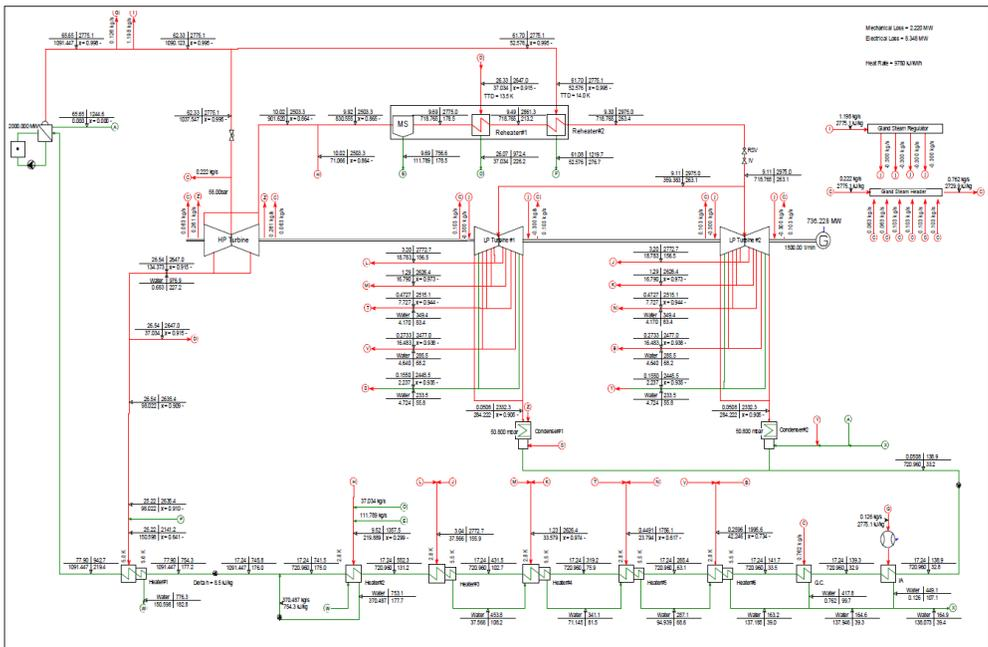
Figure 5: Heat balance diagram of NEK (Source: NEK)
