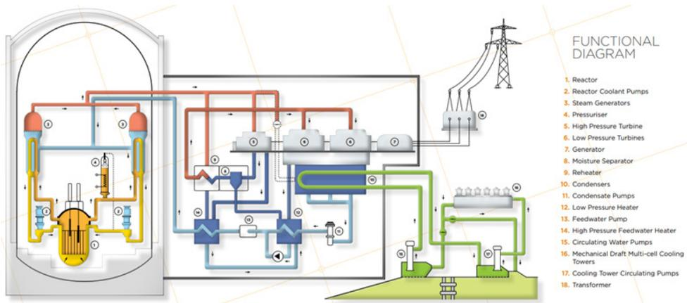
**Figure 1:** Functional diagram of NPP Krško; source: [www.nek.si](http://www.nek.si)
