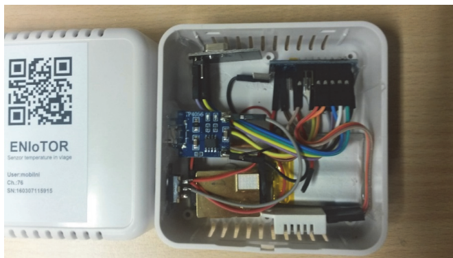
Figure 4: ENIoTOR sensor box (Source: THE4BEES project)
