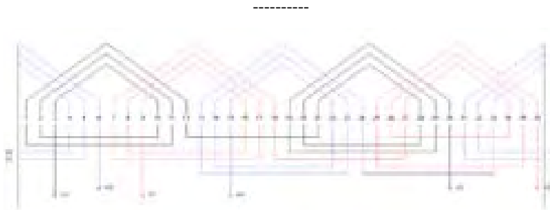
Figure 4: Stator single layer concentric winding with coil pitch 1–8, 10, 12, [3].
