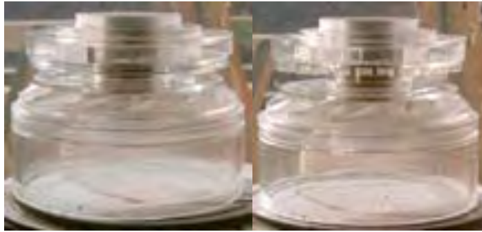
Figure 6: Centrifugal and centrifugal vortex pump stage made of Plexiglas for experimental research
