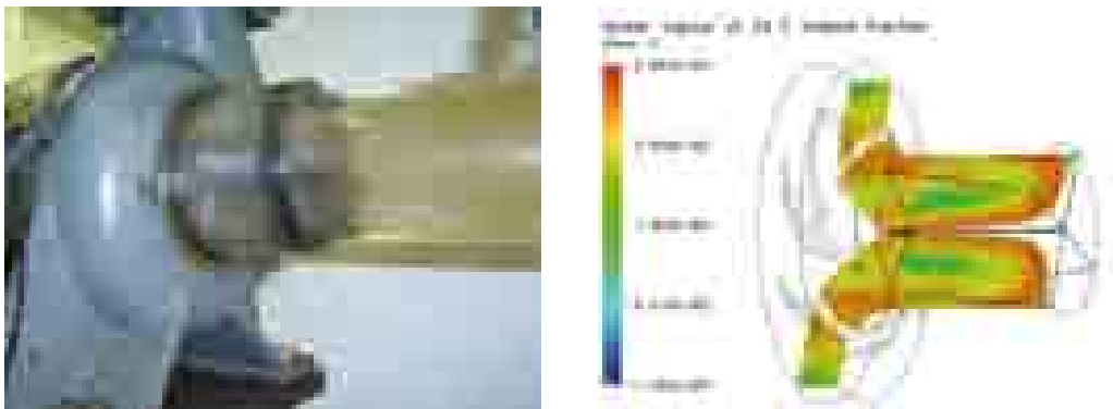
Figure 13: Hydro-dynamically induced cavitation surging on inlet geometry with guiding device.
